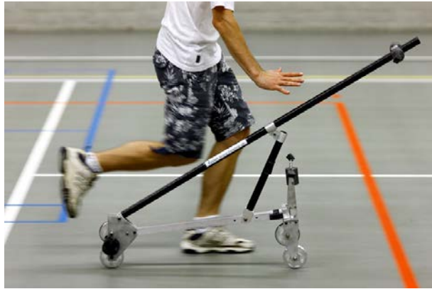
Figure 3. Two-mass-skate bicycle, a selfstable bicycle without gyros and trail [9,10].
