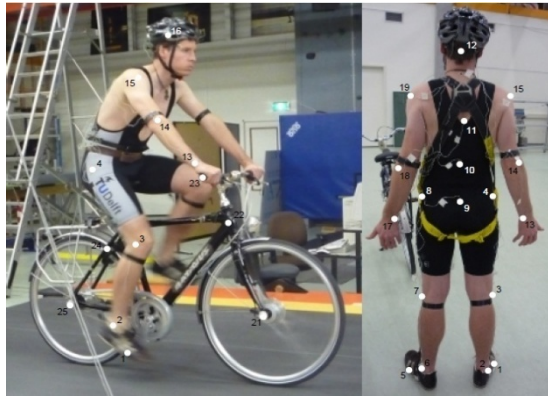
Figure 4. Instrumented bicycle and rider for rider control observations and measurements. Positions are measured with an active marker system and the bicycle is ridden on a large treadmill at the Free University Amsterdam. [11].
