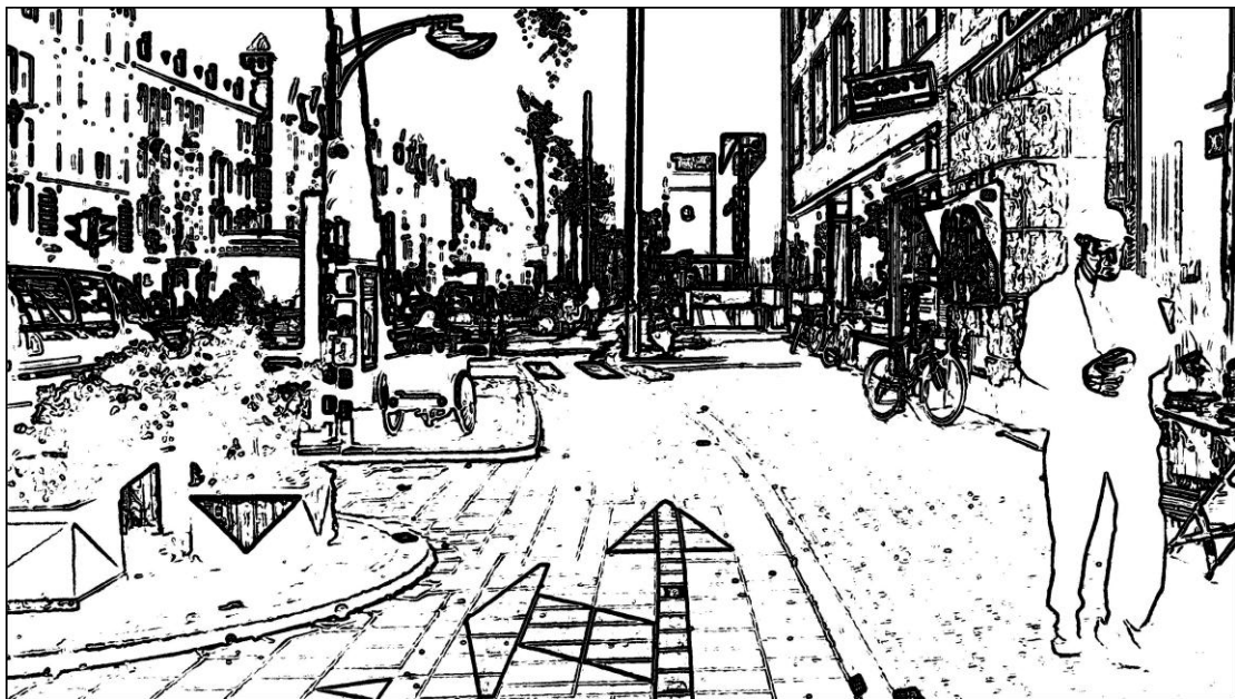
Figure 4(b). Result of the IDED-analysis of the photograph in figure 4(a) that is blurred to a level of acuity of 0.5 (only contrast differences above 0.15 are shown)
