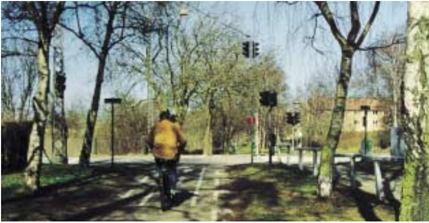
The signal is activated by detectors below the path surface, so cyclists rarely have to stop.
