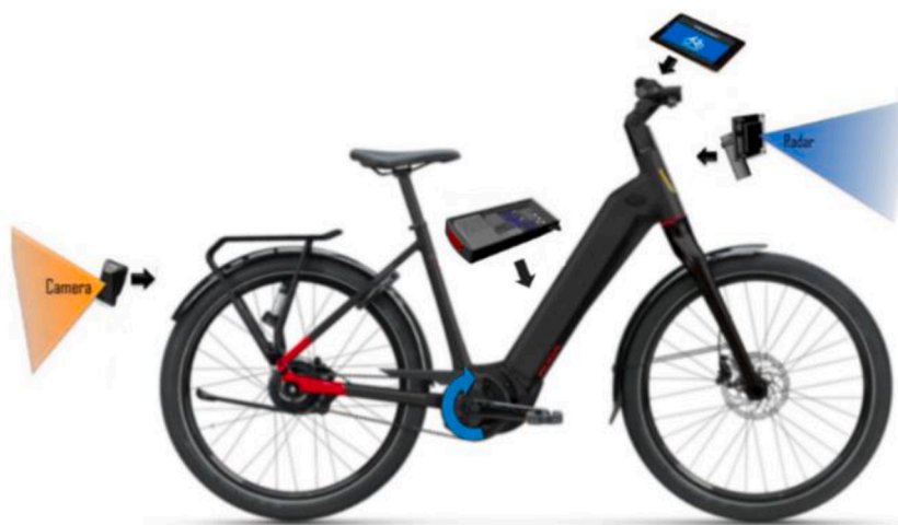
Image 1. Graphical representation of a Smart e-bike.
